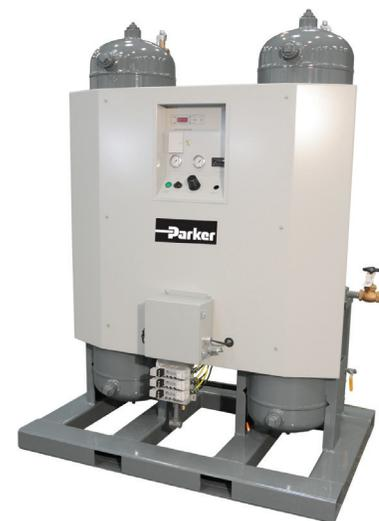
**A pressure swing adsorption (PSA) generator such as the Twin Tower Gas Generator produces up to 99.99% pure, compressed nitrogen at dewpoints to -58 degrees F (-50 degrees C).**
