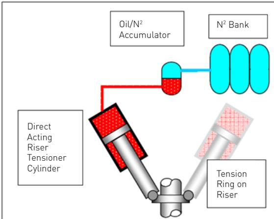
Figure 2. Sketch of direct acting tensioner cylinder.\*
