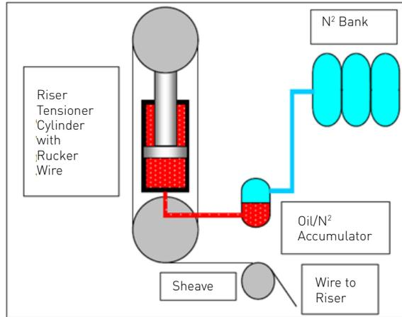
Figure 3. Sketch of conventional riser tensioner cylinder.\*
