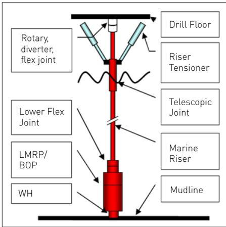
Figure 1. Schematic of a marine riser and riser system. Direct acting tensioner cylinders.\*
