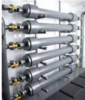
Parker Hi-Fluxx Air separation membranes provide the highest productivities on the market, delivering high N2 flow rates in a compact configuration.
