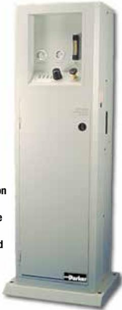
**Membrane nitrogen generators use a separation technology made up of polymer fibers that act like a membrane to remove oxygen from a compressed air stream, leaving behind clean, dry nitrogen**
